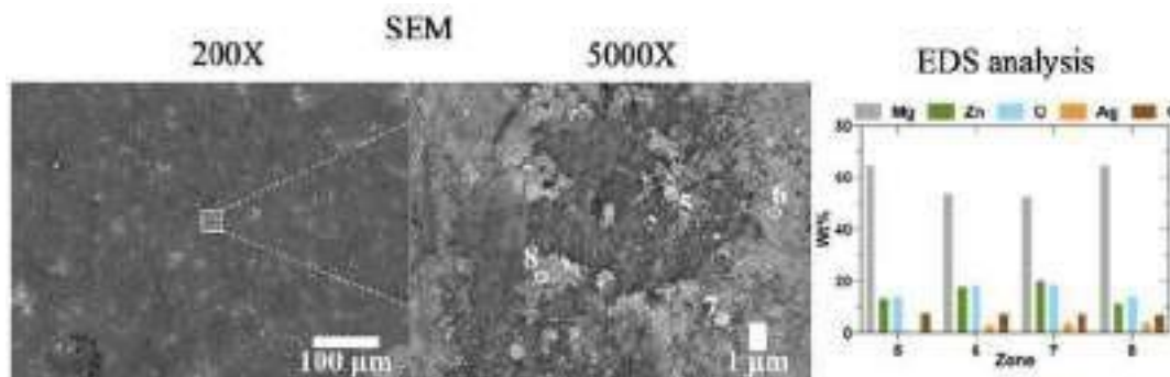
Figure 2. SEM images (200x and 5000x) and EDS analysis of electroless ZnO/Ag hybrid deposits achieved on ZnO/Mg-Ca0.3 surfaces obtained from aqueous solutions ( 10^{-3} M, at 21^\circ\text{C} ): (a-c) \text{ZnO}/\text{AgNO}_3 and (d-f) \text{Zn}(\text{NO}_3)_2/\text{AgNO}_3 .
